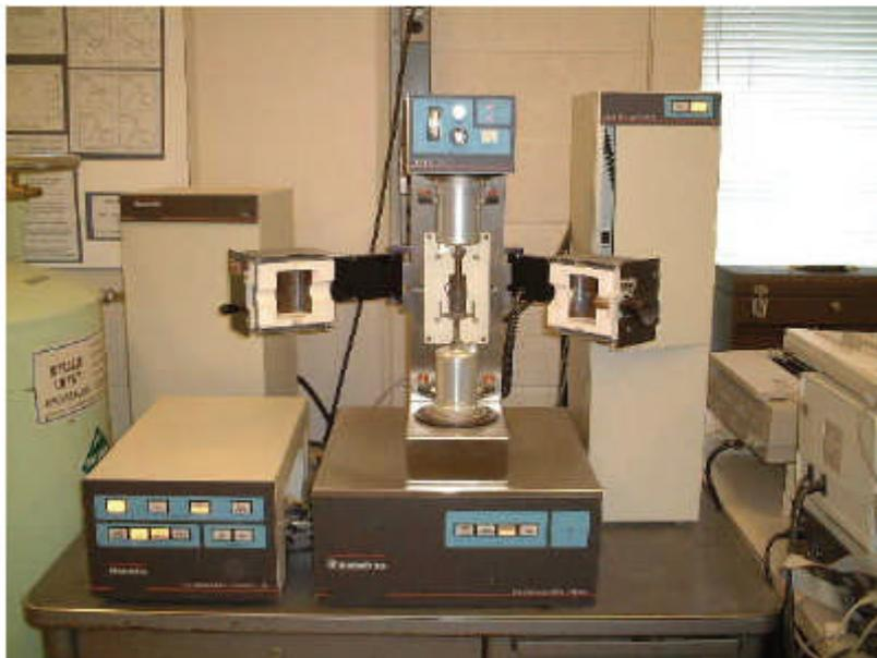
fig III-1 Appareil Rheometrics RSA-II [12]
