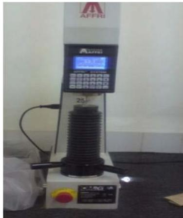
**Figure-VI -1** durometre digital
