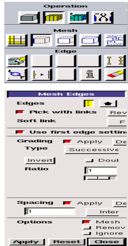
Figure III.4 : Le maillage des segments (GAMBIT Command Reference Guide, 2000).
