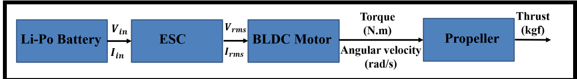
Figure 3.12: Propulsion system's power transmission process
