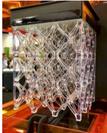
Figure III.2 Some SLA methods print parts upside down as they are pulled from the resin [101]
