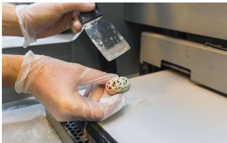
Figure III.12 A binder projection part after removing the printing powder [95]
