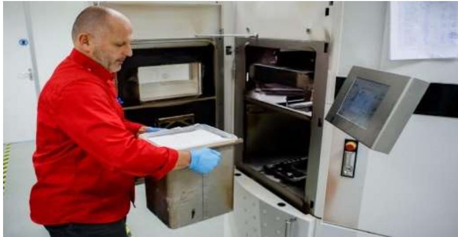
Figure III.14 Powder pin removal from the SLS process with the printed parts still enclosed in the unsintered powder [120] [101]
