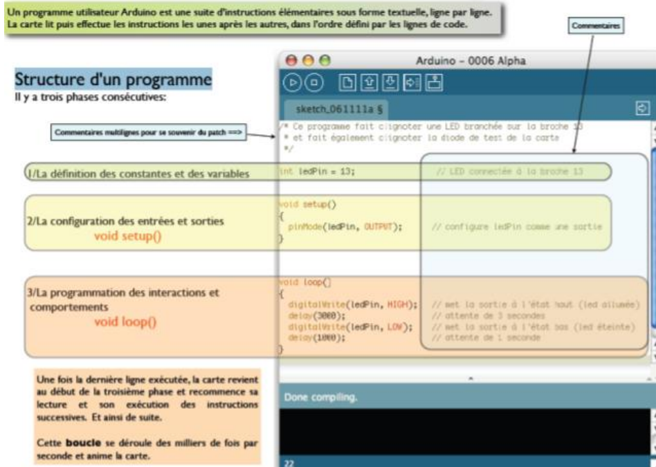
Figure 4.9: Structure d'un programme Arduino [90]
