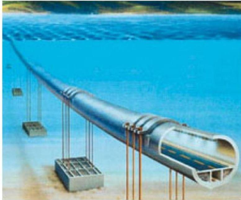
Figure 1.7 Tunnel flottant submergé (Wallis, 2010)
