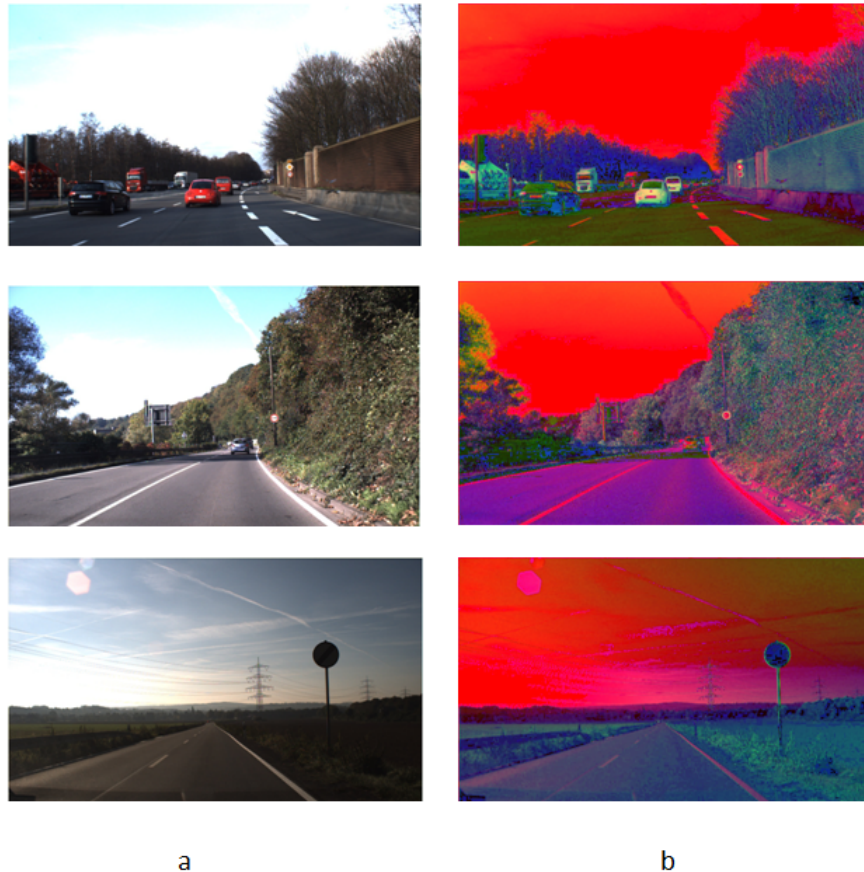
FIGURE 3.6 – Les images converties en espace HSV, (a) image RGB, (b) image HSV.
