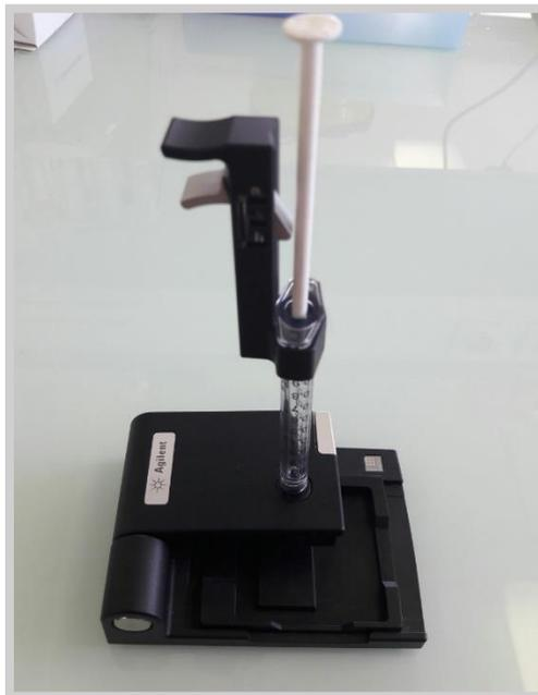
**Figure 1:** Seringue du kit Bio-Analyzer system
