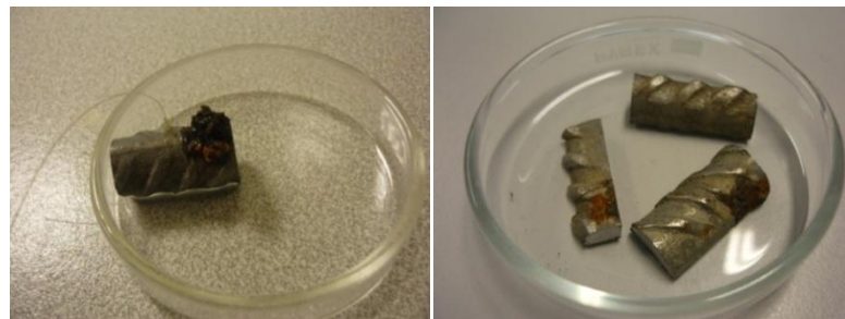
Figure III. 13 Surfaces corrodées des aciers d'armatures
